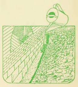
trench 6 to 8 inches wide and a few inches deepnext to the walls or piers, taking care not to go below the top of the footing. If the land slopes or the footing is more than 12 inches deep, make crowbar, pipe, or rod holes about an inch in diameter and a foot apart, from the bottom of the trench to near the footing. This will help to distribute the chemical evenly along the wall.
